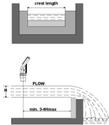
Figure 25: Rectangular Suppressed Sharp-Crested Weir
