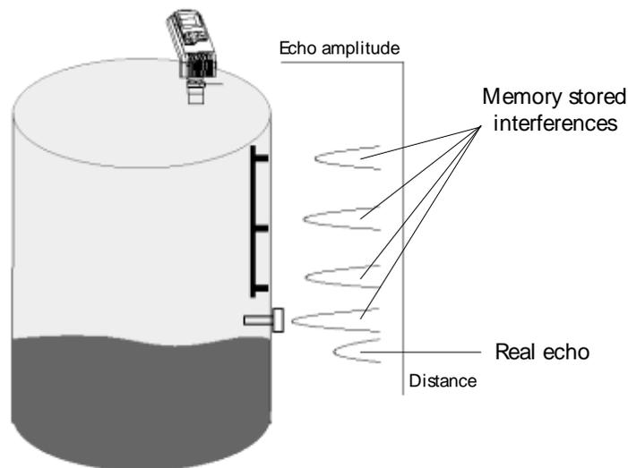
Figure 13: Scan Distance Process
