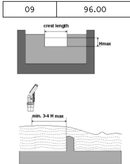
Figure 26: Rectangular Contracted Sharp-Crested Weir
