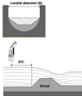
Figure 30: Palmer Bowlus Flume Trapezoidal Throat Cross-Selection
