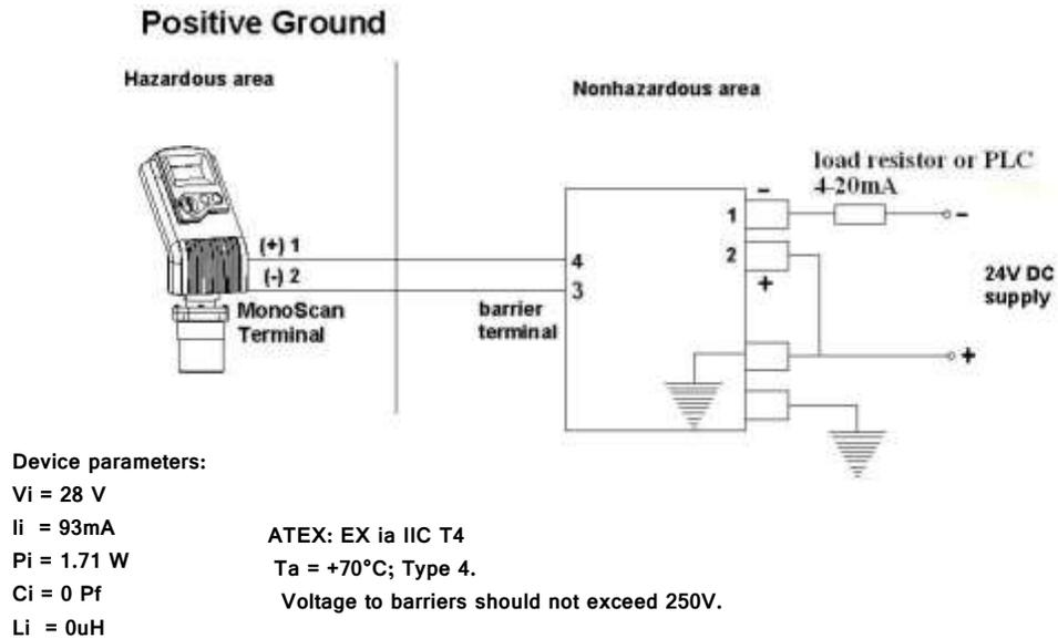
Figure 9: Intrinsically Safe Positive Ground Connection
