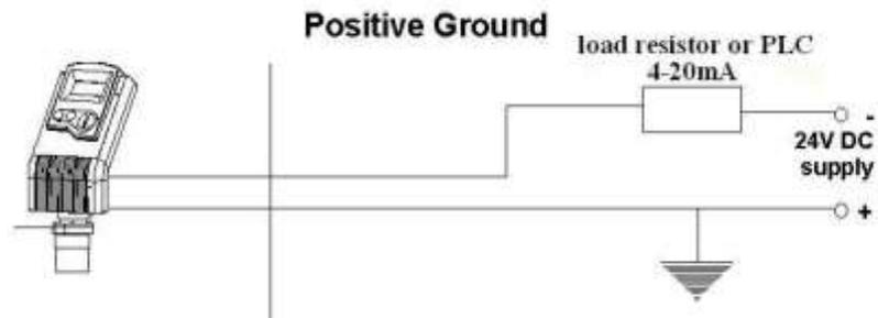
Figure 7: Non-Intrinsically Safe Positive Ground Connection
