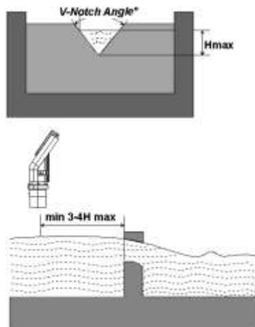
Figure 28: V-Notch (Triangular) Sharp-Crested Weir
