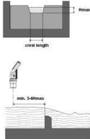
Figure 27: Trapezoidal (Cipolletti) Sharp-Crested Weir
