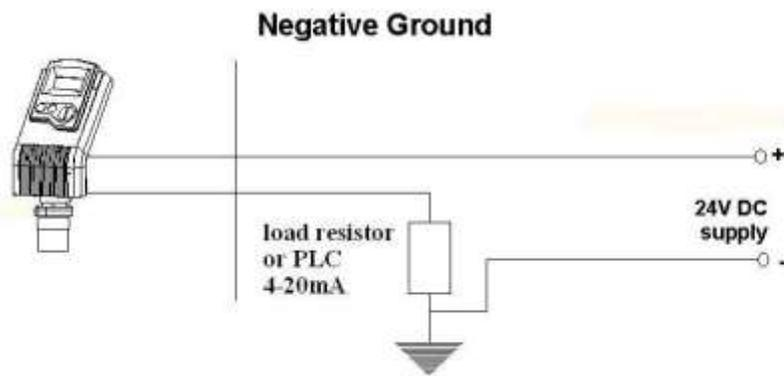
Figure 8: Non-Intrinsically Safe Negative Ground Connection
