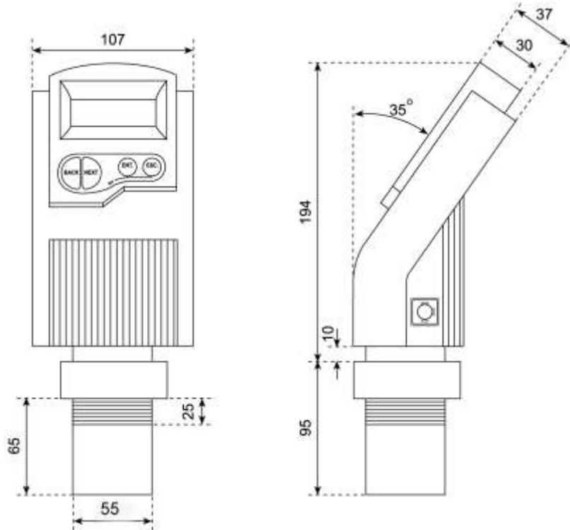
Figure 1: Front View of MonoScan    Figure 2: Side View of MonoScan
