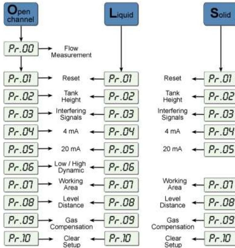
Figure 11: MonoScan Functions Menus
