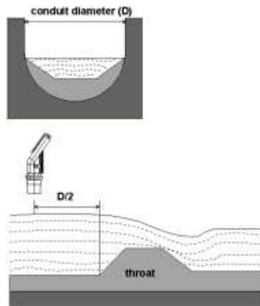
Figure 10: Palmer Bowlus Flume Trapezoidal Throat Cross-Selection
