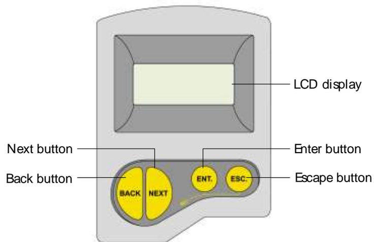
Figure 12: MonoScan Display and Function Buttons
