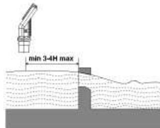
Figure 17: V-Notch (Triangular) Sharp-Crested Weir
