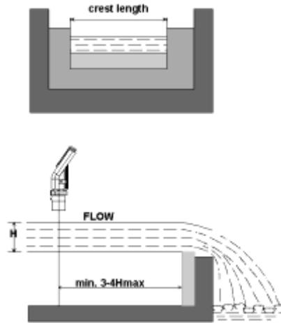
Figure 14: Rectangular Suppressed Sharp-Crested Weir
