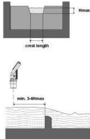
Figure 16: Trapezoidal (Cipolletti) Sharp-Crested Weir
